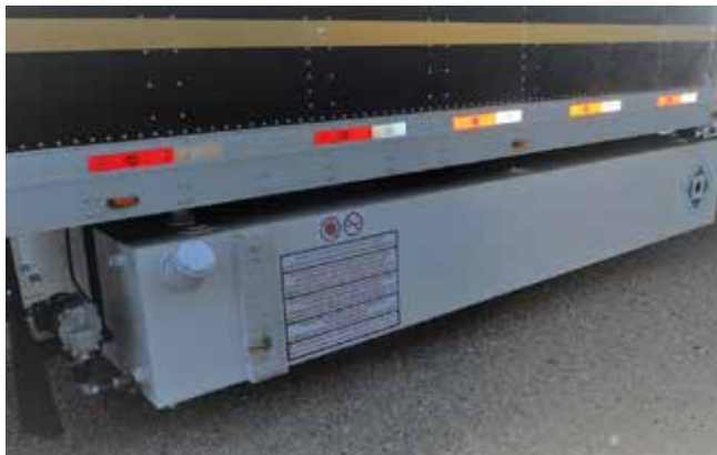
7774 liter Double walled U/S fuel tank c/w locking filler cap-fuel level indicator and pump.
