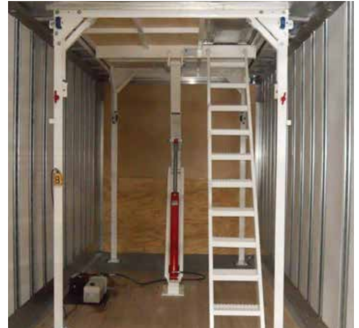
Remote control hydraulic scissor lift, 12V power pack with trickle charger.
